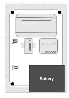
5 - Attach the negative (6) and positive (5) terminals to the battery with the supplied screws and washers (inside the accessory pack attached to the battery leads) NOTE only use LIFePO4 batteries as this is what the charge controller has been programed to charge, It is **not** suitable for Lead Acid Batteries
