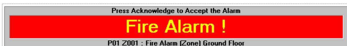
In order to provide clear and unambiguous alarm information, easily recognised by the operator all alarm types are displayed, throughout the MAESTRO system by different colour codings. In the quiescent state, with no alarms current, the alarm banner is displayed in a grey colour, on the receipt of an alarm message the banner changes as follows.
