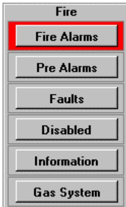
By left hand click of the mouse cursor on any of the active Fire Alarms buttons, a listing of all current alarms in the system is displayed.
