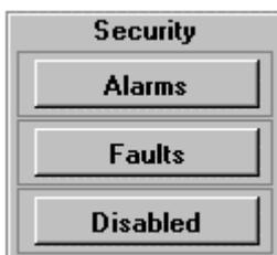
By left hand click of the mouse cursor on any of the active Security Alarms buttons, a listing of all current alarms in the system is displayed.
