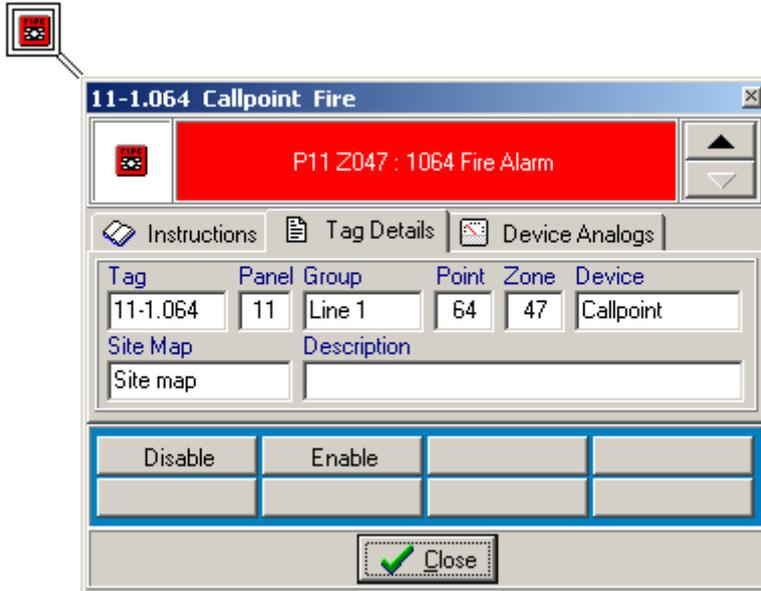
Information cards are programmed at the system configuration stage, with separate information for different alarm conditions. The following illustration shows a zone information card for both normal and fire condition.
