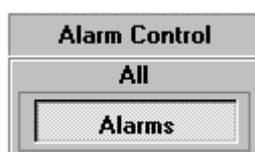
For example, if a fire alarm and fault condition occur simultaneously the All Alarms button will display a red boarder, as MAESTRO gives fire the highest priority. If the fire condition is subsequently cancelled, the boarder of the All Alarms button will change to a yellow colour, as fault is now the highest alarm priority.
