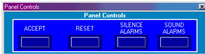
In multi panel systems, all operations made from the panel controls display buttons are global, that is all panels connected to MAESTRO are effected by the action.
