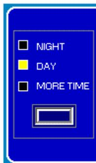
Daytime settings are usually applied to the panel when buildings are occupied, or 'manned'. Settings may include such facilities as alarm delays for evacuation programmes, or changes of sensitivity of specified sensors.
