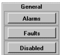
By left hand click of the mouse cursor on any of the active General Alarms buttons, a listing of all current alarms in the system is displayed.
