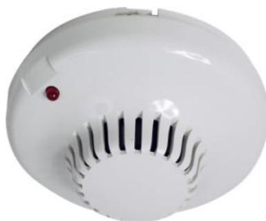
In the ionization type, charged particles are attracted from an ionizing source across the sensor chamber to a collector. The presence of smoke particles slows the particle stream. This change in speed is detected and amplified by the sensors electrical circuits.
