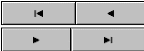
Allows scrolling through the alarm lists. Button order is First Alarm (oldest in list), Prior Alarm, Next Alarm and Last Alarm (latest in list). These buttons scroll lists by zones or points depending upon which has been selected from the toolbar. Lists can also be scrolled by zones from the scroll buttons at the ends of the Alarm Information Bar. (Section 2.5.)
