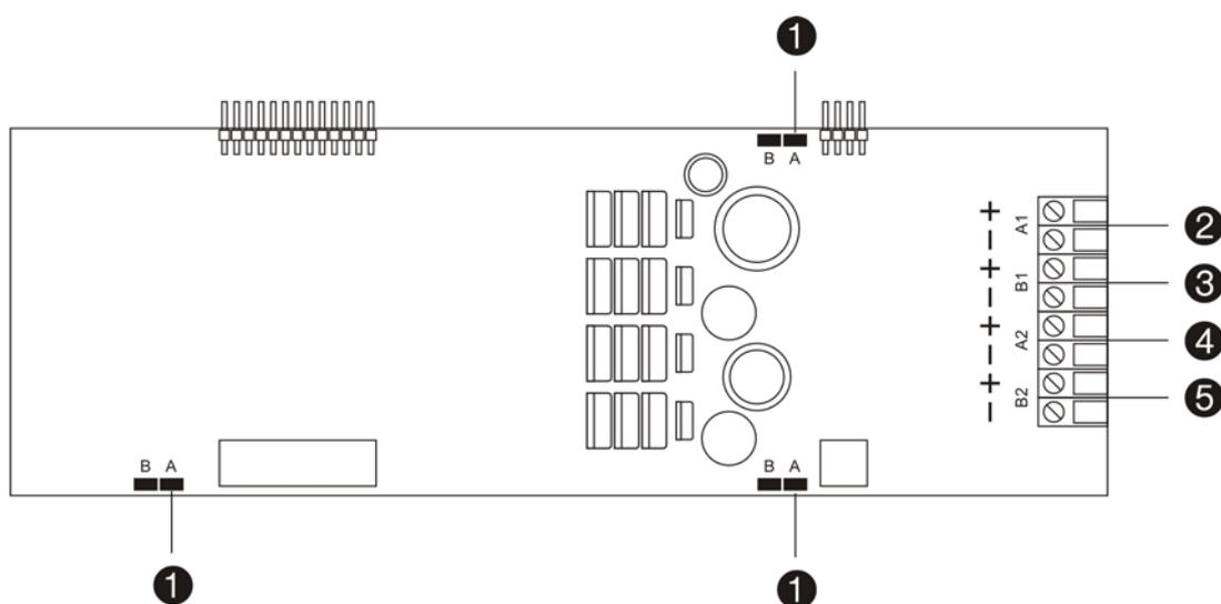
1. Loop Class configuration jumpers A and B
