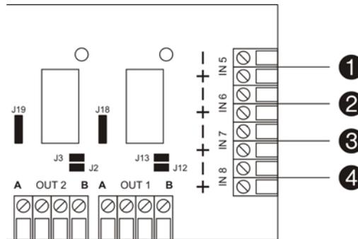
1. IN5 general input OR fault routing return input (VdS mode)
