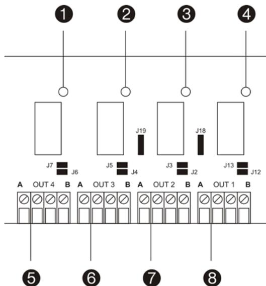
1. OUT4 fault routing output LED
