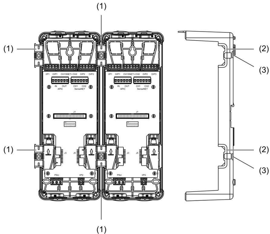
1. Joining clips (front view)
