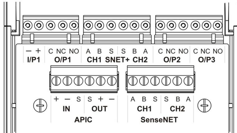
Figure 13: Backplane PCB connectors (bottom)
