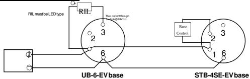
Auxiliary terminal RIL current limited to 3mA. Base control is not current limited as the auxiliary equipment provides the limiting. If the +ve supply for the auxiliary equipment is taken from the EV loop, care must be taken to not cause corruption of the EV protocol by excessive current draw.
