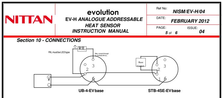
Auxiliary terminal RIL current limited to 3mA. Base control is not current limited as the auxiliary equipment provides the limiting. If the +ve supply for the auxiliary equipment is taken from the EV loop, care must be taken to not cause corruption of the EV protocol by excessive current draw.
