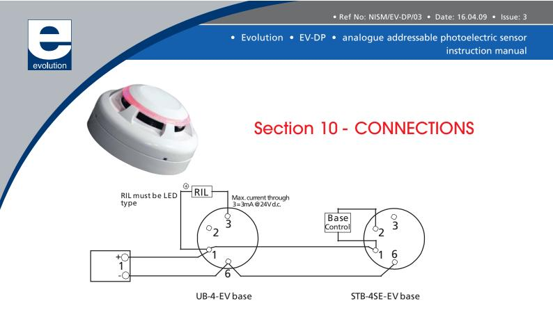
Auxiliary terminal RIL current limited to 3mA. Base control is not current limited as the auxiliary equipment provides the limiting. If the +ve supply for the auxiliary equipment is taken from the *EV* loop, care must be taken to not cause corruption of the EV protocol by excessive current draw.
