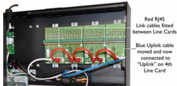
Figure 2.9 — Console with Four Line Cards Fitted
