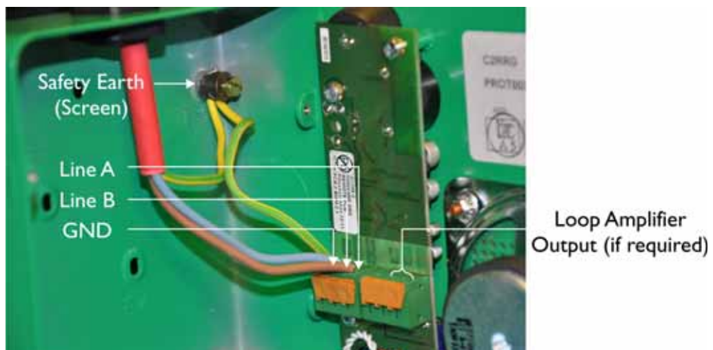
Figure 2.31 — DRS Refuge Remote Connection Details
