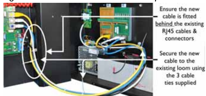
Figure 2.15 — Recommended cable tie positions
