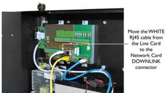
Figure 2.22 — Network Downlink Connection
