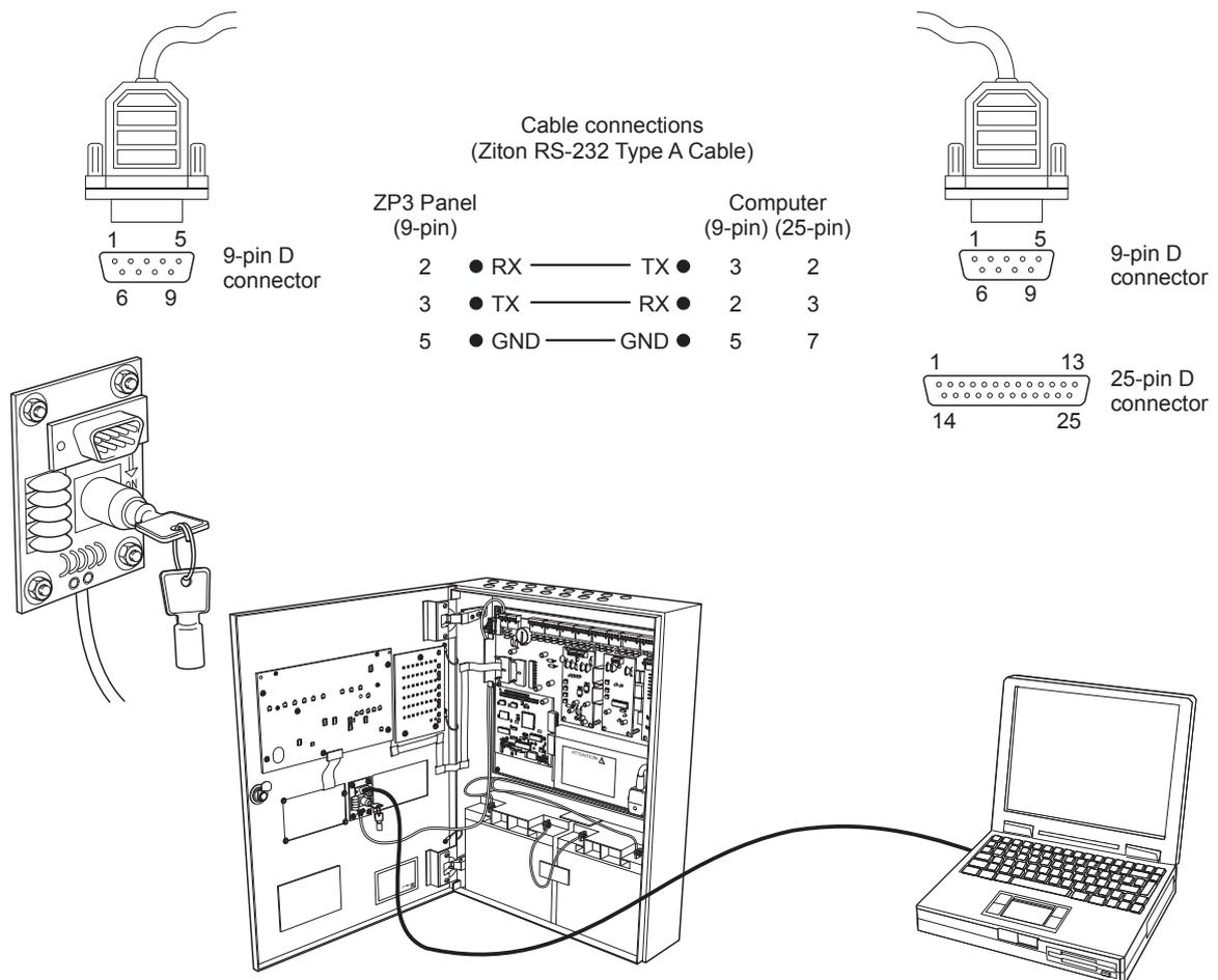
RS-232 is officially specified as having a maximum cable length of 10 metres, which is more than adequate for ZP3/PC configuration functions. The connecting cable must be screened, and must be made-up as per Figure 10. Alternatively, a standard null modem cable can be used.
