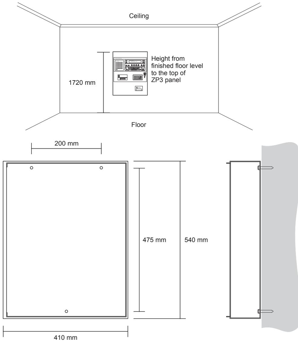
Use appropriate mounting screws such as plastic rawl plugs, expansion anchors, etc., depending on the type of wall. Use M4 screws at least 20 mm long. The mounting system must be able to support a minimum weight of 20 kg, which is the total weight of the panel (with batteries).
