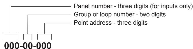
The ZP3 panel incorporates one control bus with 1,024 addresses that can be either inputs or outputs. Refer to the “System address list” on page 97 for details. These addresses are divided into two groups, system bus and user bus, as shown in the following table.
