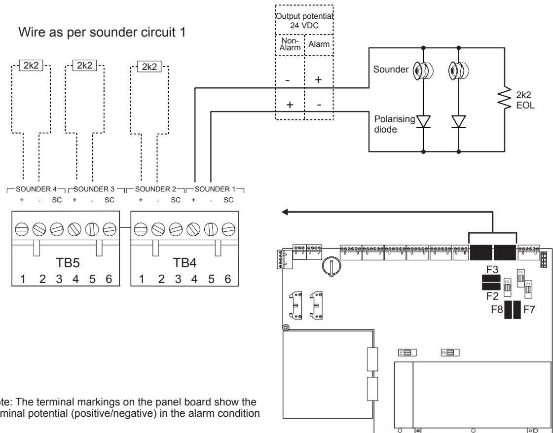
Sounders connected to the circuits must be polarized, i.e. fitted with diodes so that they operate with power in one polarity direction, and not in the reverse direction.
