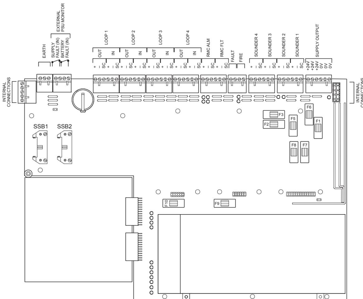
**Note:** All terminals accept wiring sizes from 0.5 mm<sup>2</sup> to 2.5 mm<sup>2</sup>.
