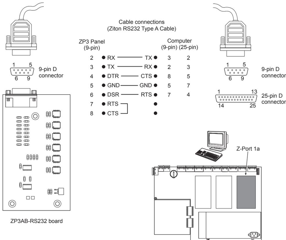
RS-232 is officially specified as a maximum cable length of 10 metres. However, if slower baud rates are used, then it is possible to operate it at up to 50 metres. Cable must be screened, with at least five conductors, and must be made up as shown in Figure 13.
