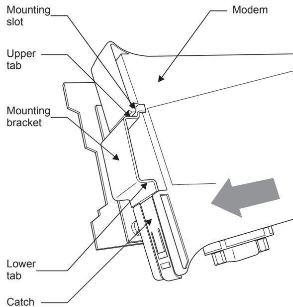
**Figure 23: Installing the accessory plate and connecting the RS-232 and power cabling**
