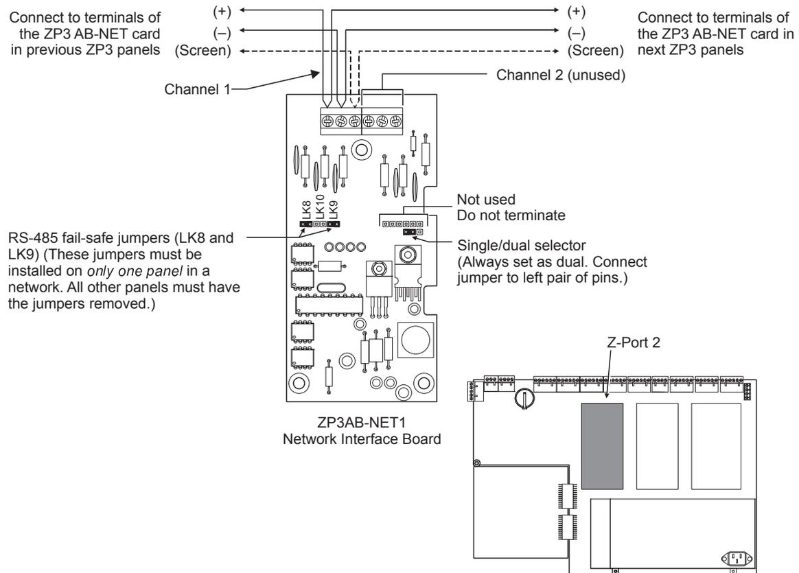
RS-485 operates through up to 2,000 metres of screened, twisted-pair cable. Wiring can be daisy-chained point-to-point, or can be T-tapped or spurred for short distances i.e. less than 10 m. The total length of cable in the network should not exceed 2,000 metres. If the network distances are greater than 2,000 metres, use RS-485 booster units, or fibre-optic cable. For more information refer to the *ZP3AB-NET1 Network Board Installation Sheet* (P/N 501-0485ZE-1-01).
