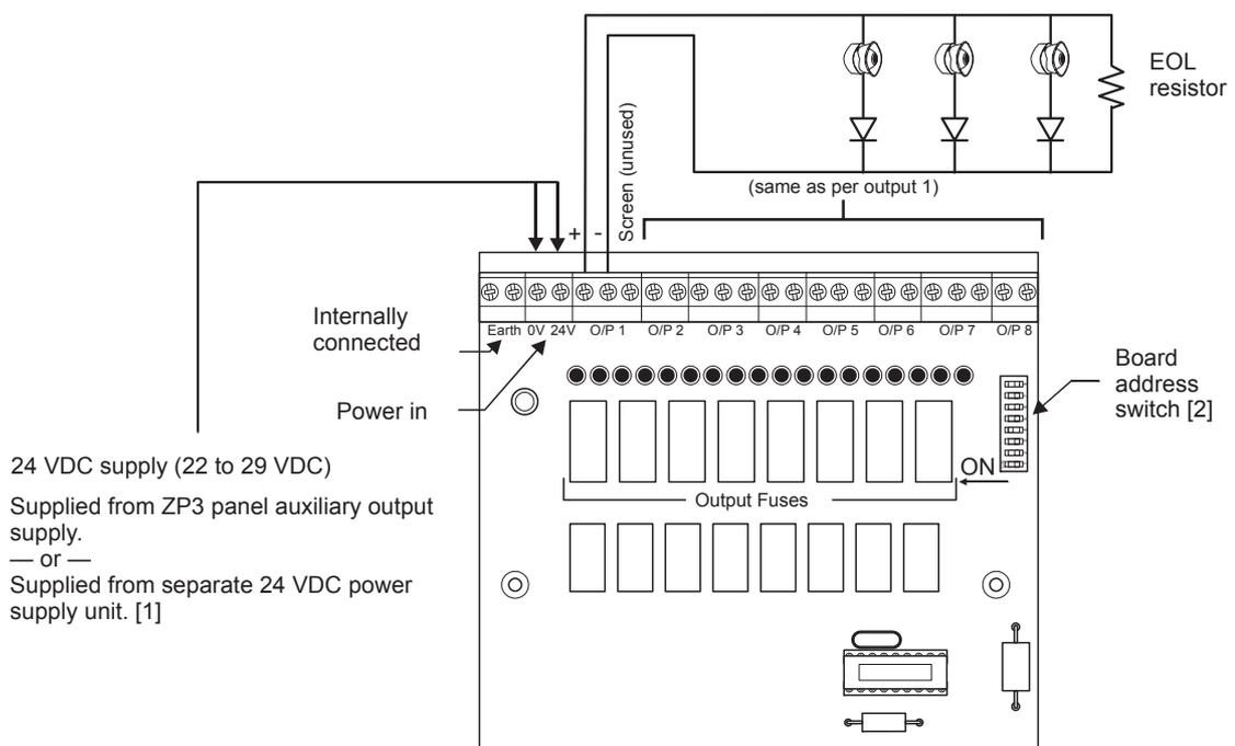
[1] If externally supplied, do not common the power supplies, i.e. do not connect the 0V of the internal and external power supplies together.
