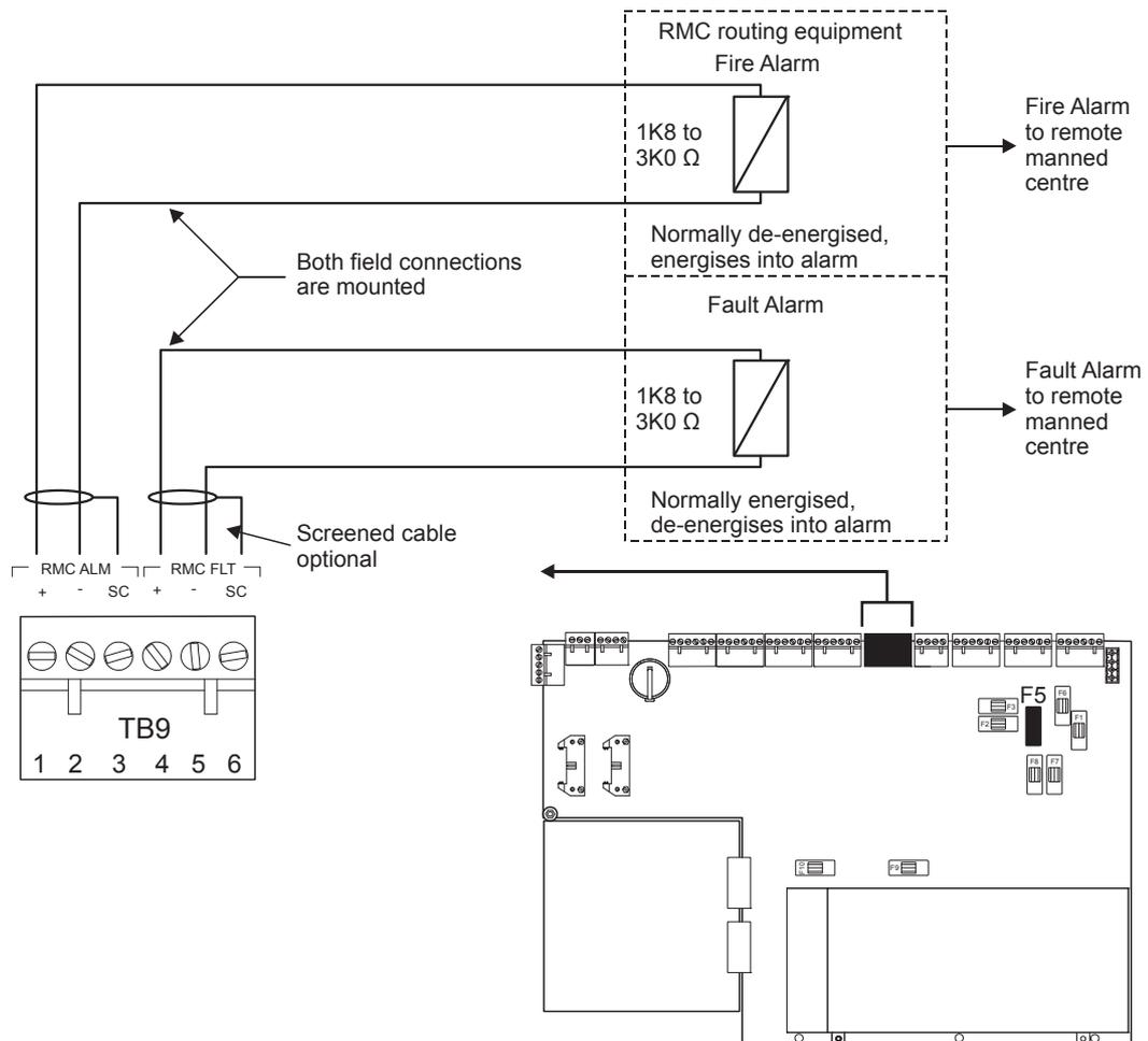
The RMC outputs are designed to drive relays in the fire alarm routing equipment. These relays must have a coil resistance of 1.8 to 3.0 kΩ.
