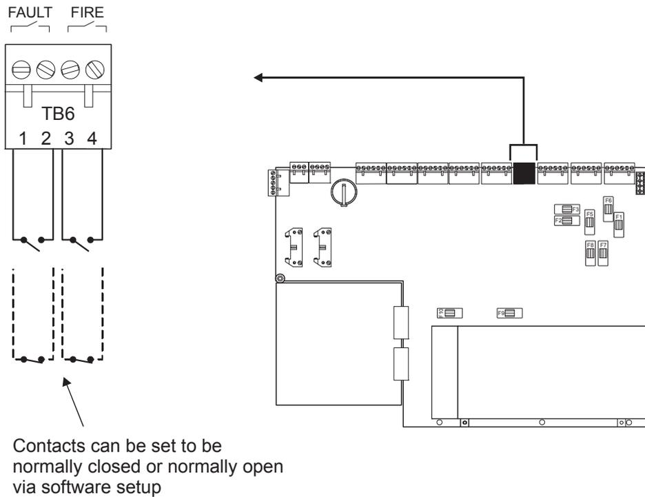
The relay contacts are rated for a maximum current of 1 A, and a maximum voltage of 24 VDC or 100 VAC.
