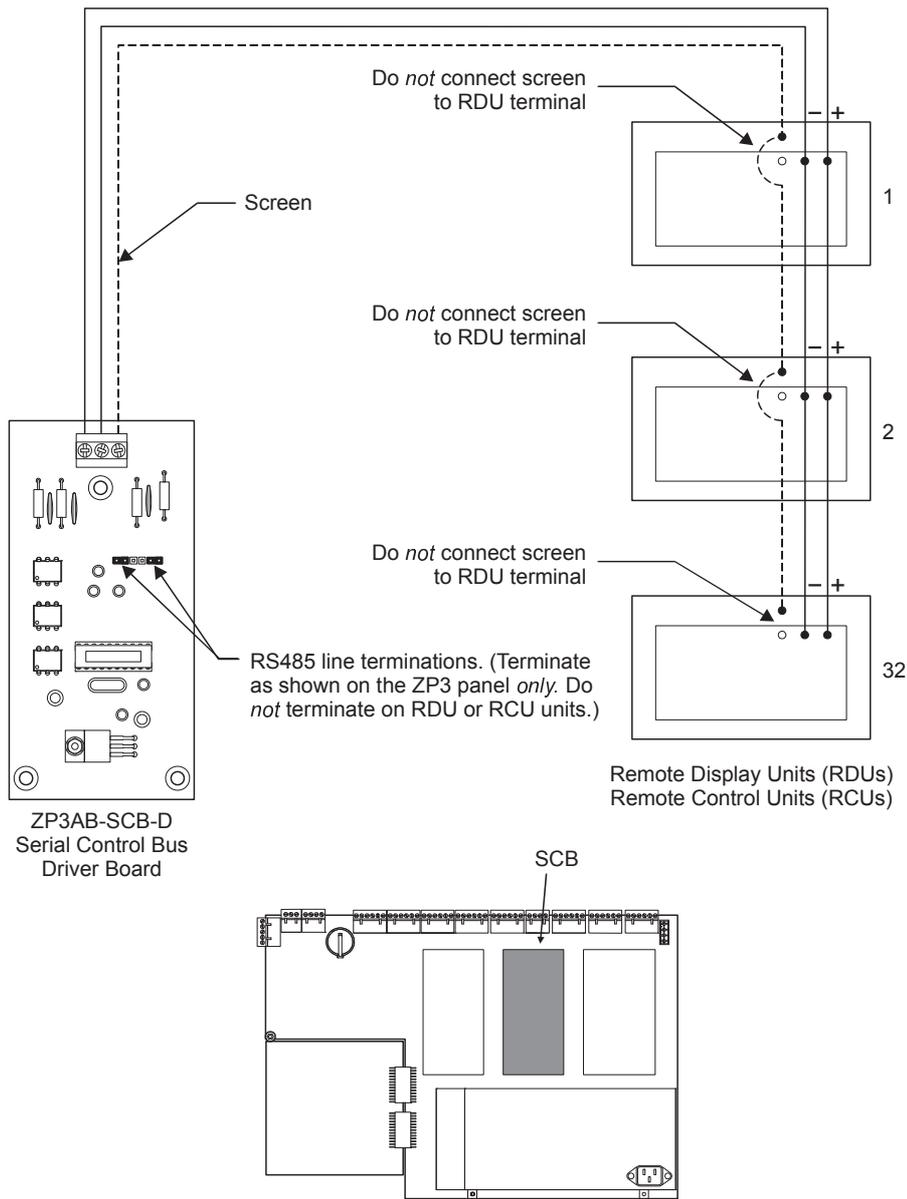
**Note:** The RDU screen must *only* be connected on the ZP3AB-SCB1 Serial Control Bus Driver Board in the ZPR Panel. The screen must *not* be connected at the RDU.
