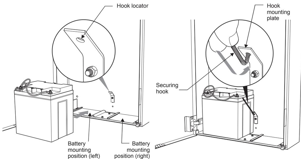
**Figure 36: Securing the backup batteries**
