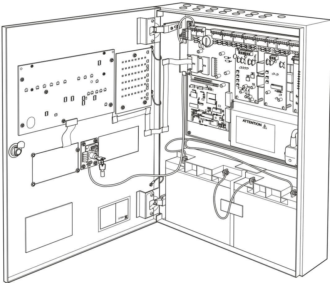
Figure 4 shows the basic fire panel. The elements shown provide all required functions, and form the core of the ZP3 panel. No optional I/O modules or printer are shown in this illustration. Three communication boards are fitted.
