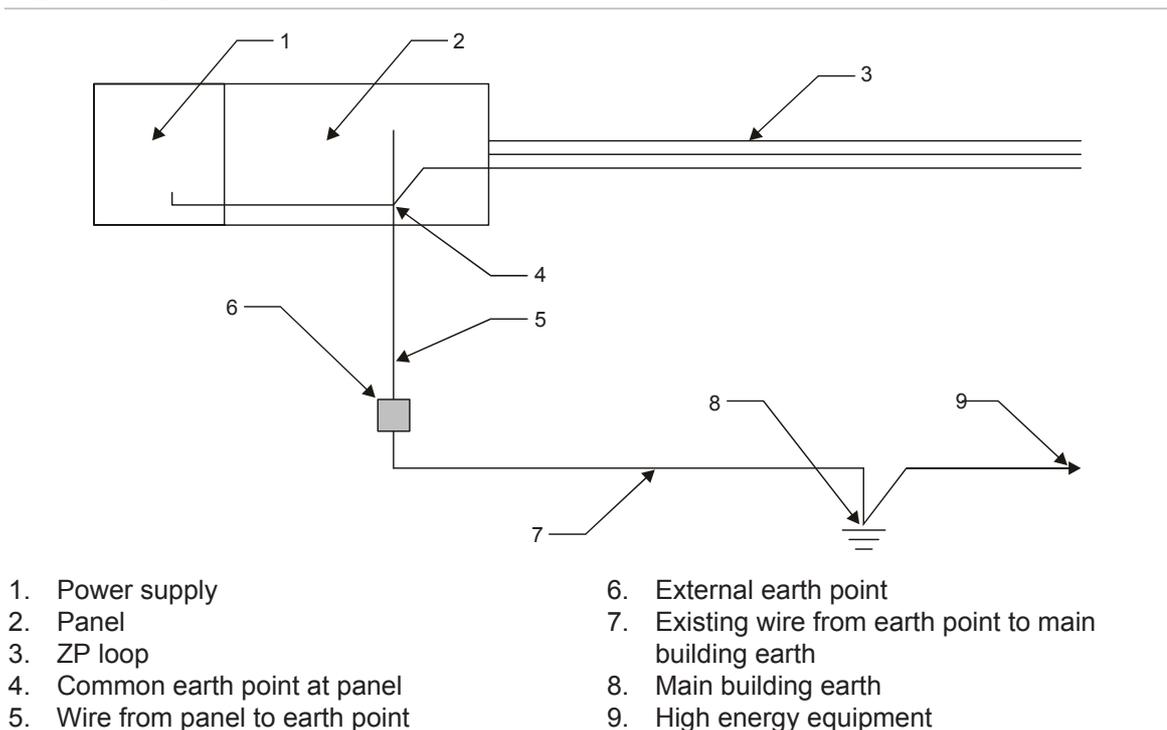
The wire from the panel to the external earth point should be at least 4 mm<sup>2</sup> cable and be securely connected at both ends to ensure a good mechanical and electrical connection. Use crimped lugs where possible.
