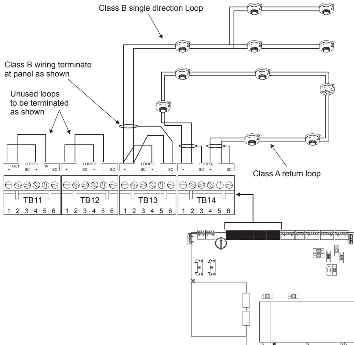
When wired in Class B single direction format, then the loop terminals must be connected (+) in to (+) out and (-) in to (-) out.
