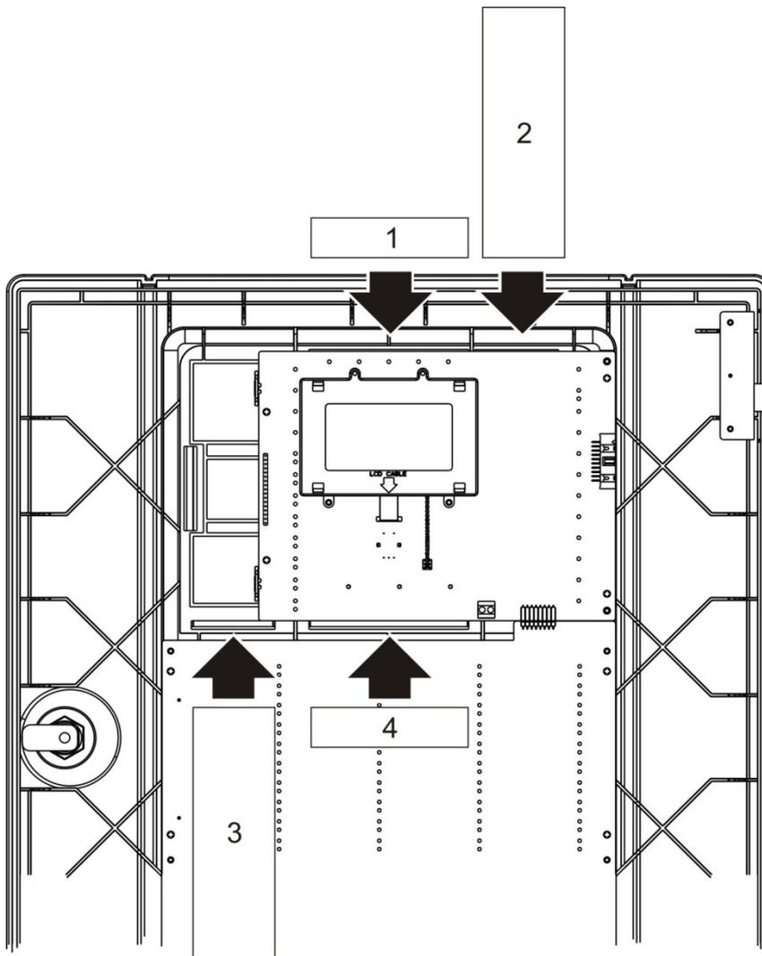
The inserts are numbered 1, 2, 3, and 4, and are inserted at the location indicated (with the printed area facing the front of the control panel).
