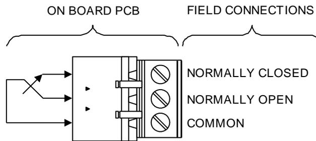
The fault relay is derived from a single pole change over 'volt-free' relay contact which is not fault monitored. The maximum contact current rating is 2A @ 24V DC. Inductive loads should be diode protected to prevent back EMF causing damage to the relay contact.
