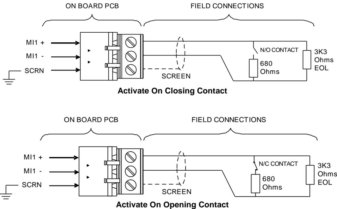
**Note:** When a monitored input is configured as a normally closed extinguishant flow input, connecting a normally open switch will cause the panel to go into a release state. Likewise when a monitored input is configured as a normally open extinguishant flow input, connecting a normally closed switch will cause the panel to go into a release state.
