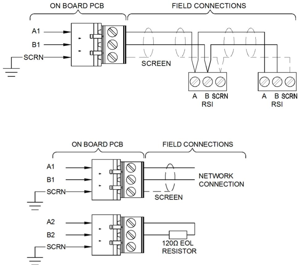
These ports on the panel are for connections to a Remote Status Indicator (RSI) device (Maximum 8 devices). This is an RS-485 connection operating at 57.6 kbps.
