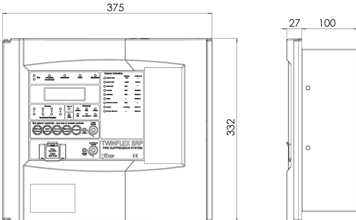
The control panel back box is designed as a dual-purpose surface or flush mount unit.
