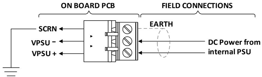
DC power from the internal system power supply. 31V DC, 5A rating.
