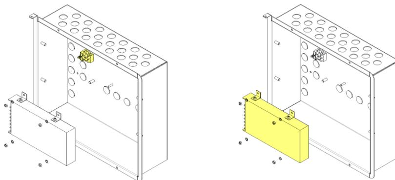
The control panel requires standby batteries. Fike recommends 2 x Yuasa YUCEL Y12-12 or equivalent. The sealed lead acid batteries should be installed according to the following diagram. These are to be sited in the control panel back box using the provided clamps. The batteries should be connected in series using the connection leads supplied. See the section entitled *Control Panel Connections* for panel connections.
