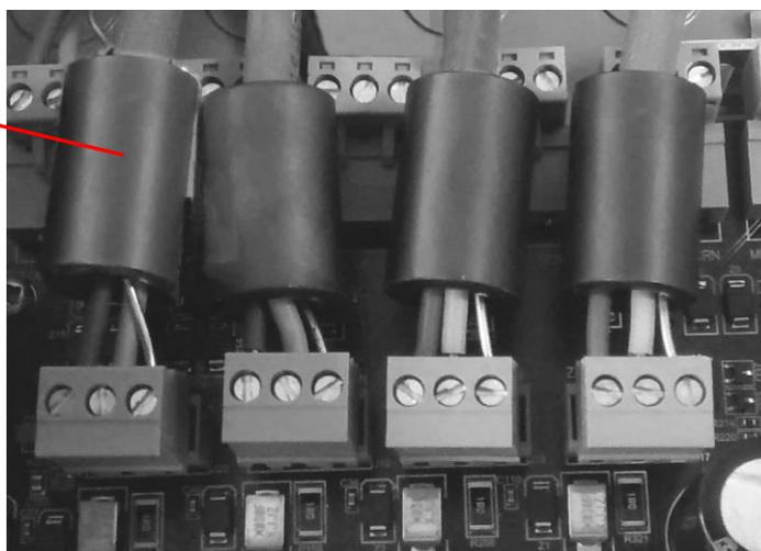
2. The cable screen must be connected to the SCRN terminal for each circuit at the control panel only.
