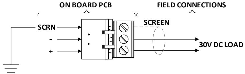
An auxiliary nominal 31V DC power supply is available to power ancillary devices requiring up to 30V DC. Each auxiliary output can be programmed to cycle power during a system reset, or to keep its power constant during a system reset.
