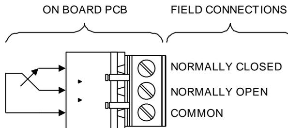
The relays are derived from a single pole change over 'volt-free' relay contact which is not fault monitored. The maximum contact current rating is 2A @ 24V DC. Inductive loads should be diode protected to prevent back EMF causing damage to the relay contact.
