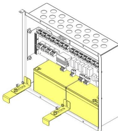
When fitting new batteries the total battery voltage must not be less than 21.5V. If the battery voltage is less than 21.5V the charger will assume that they are faulty and will not charge them.
