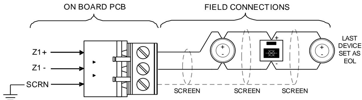
Each zone requires a separate 2-core radial circuit from the control panel to the furthest point of the zone, to a maximum of 500 meters.
