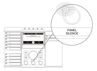
The Panel Silence LED turns on and the buzzer stops. New alarm or fault events will turn the buzzer back on.
