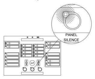
The Panel Silence LED turns on and the buzzer stops. New alarm or fault events will turn the buzzer back on.
