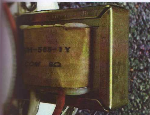
Fig. 10 The view of the transformer type H-585-1Y used in VA-565, VA-575 loudspeakers
