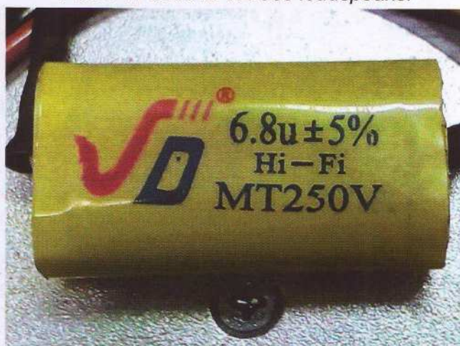
Fig. 13 The view of the capacitor type MT250V 6,8μF used in VA-585
