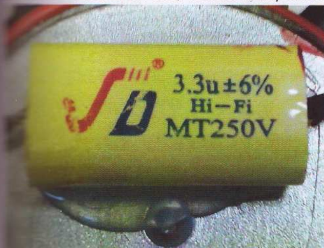
Fig. 12 The view of the capacitor type MT250V 3,3μF used in VA-565, VA-575
