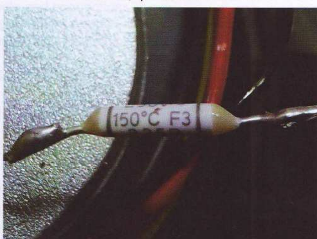
Fig. 15 The view of the thermal fuse type UMI 5A 150°C F3 225 R
