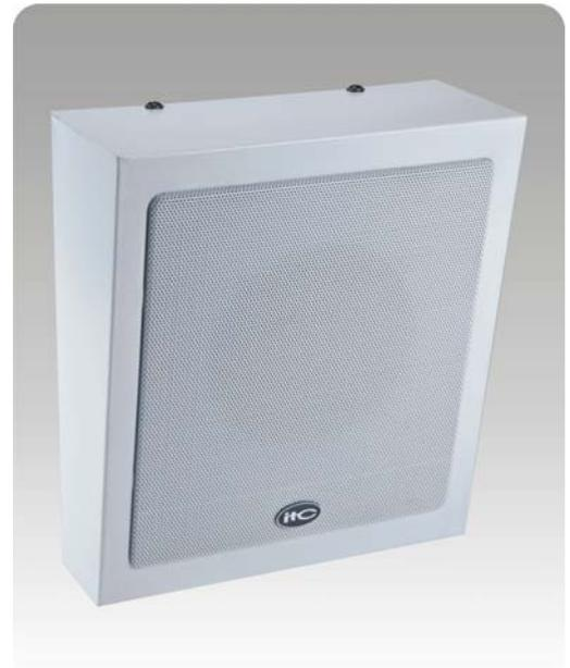
The built-in 5" full range speaker driver is designed of wide frequency response 100-16kHz, the multiple power taps 0.75W, 1.5W, 3W & 6W are helpful for different applications varies from room size and ambient noise surroundings.
