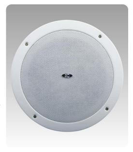
The built-in 5" speaker driver is designed of wide frequency response 110-18KHz, power output is 3w, 6w & 9w. The aluminum grille, metal baffle and metal back cover are in attractive white color.
