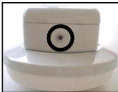
Picture 4 - the programmer's socket
