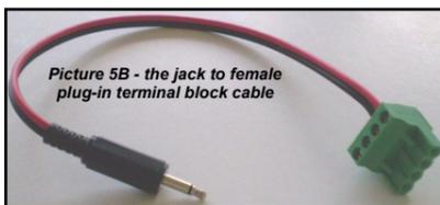
Picture 5B - the jack to female plug-in terminal block cable
