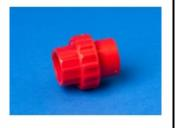
This ABS Socket Union is used for aspirating systems and is compatible with all our HSSD systems. A suitable adhesive should be used when connecting ABS pipe. The union allows you to maintain and fit the pipe easily by breaking a pipe join at a union without putting strain on the rest of the pipework.
